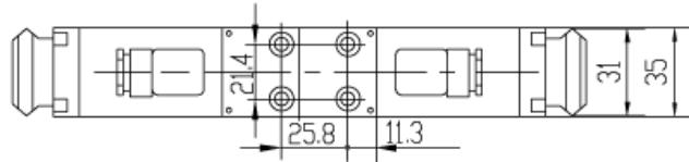
Shape and connection dimensions of 2-position valve.
