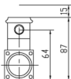
z5L large plug-in connector with indicator
