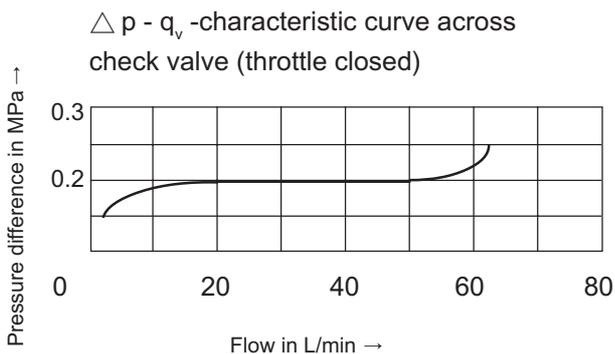
Pressure difference  $\Delta p$  in relation to the flow  $q_v$  at constant throttle setting
